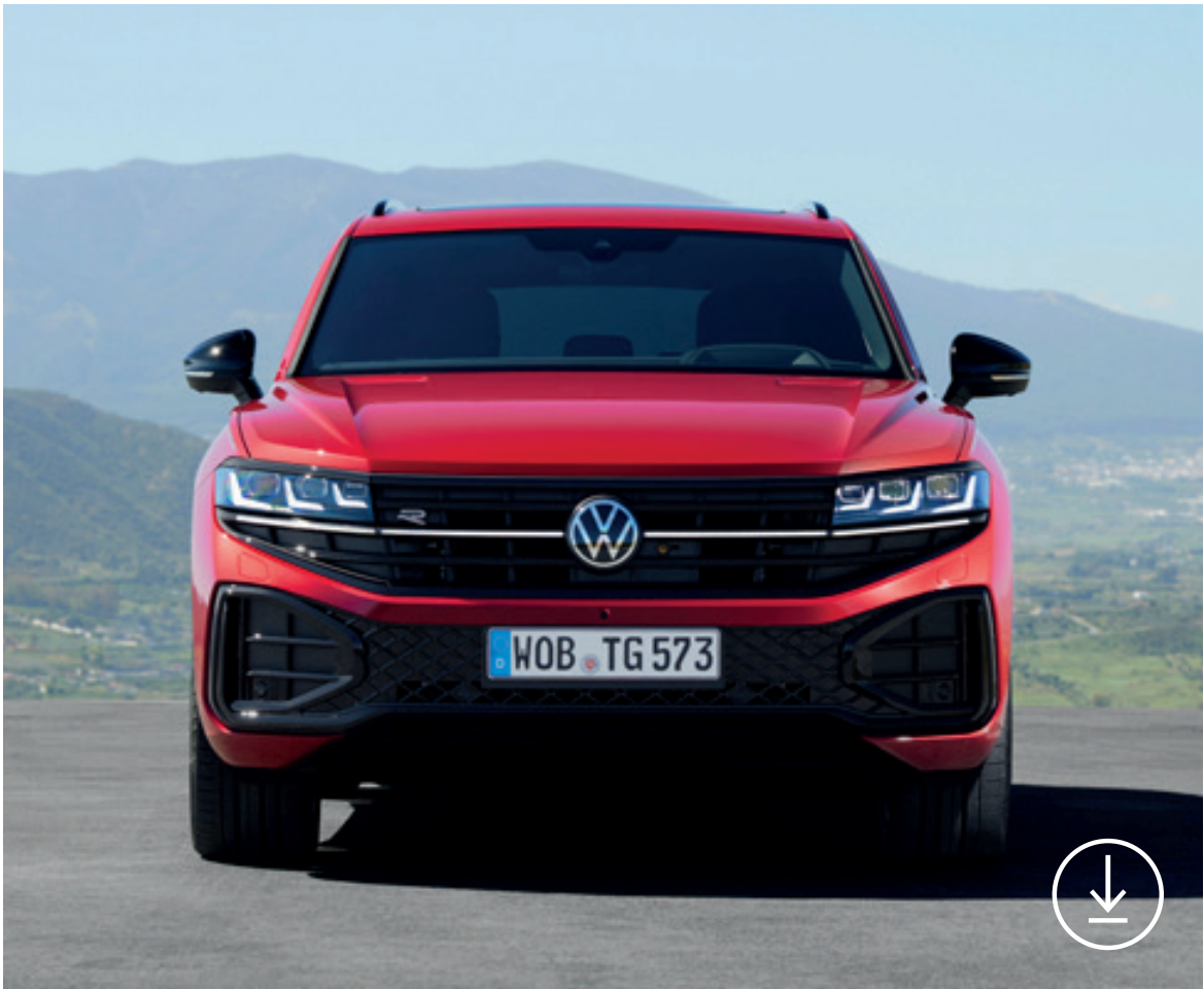
A horizontal white LED strip in the radiator grille is part of the daytime running lights of the IQ.Light HD matrix headlights.
