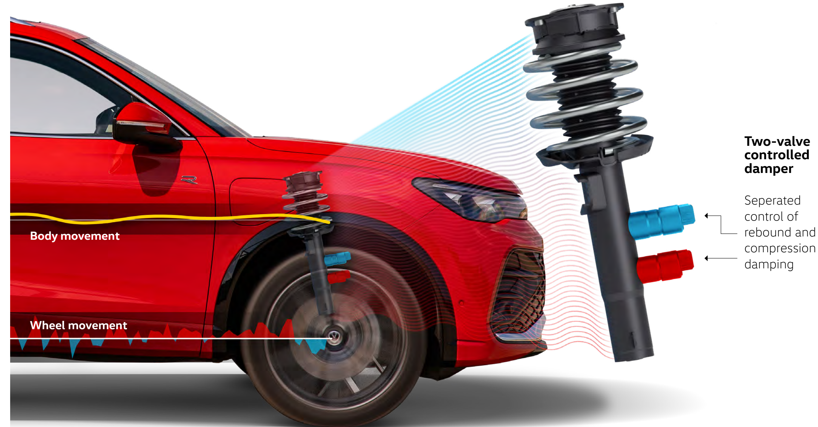
The technical structures of the adaptive DCC Pro chassis
